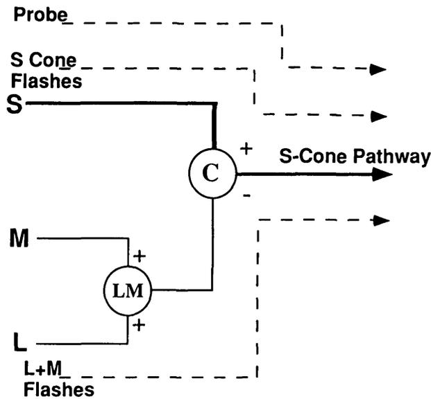
Fig. 1. The skeletal model of the initial stages of the S cone system. The S, M, and L cones act as linear transducers. The signals from the L and M cones are summed to make the LM signal. The difference between the S cone and LM signals constitutes an opponent chromatic signal (C).
