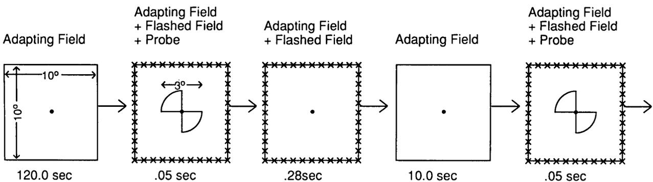
Fig. 3. The spatial and temporal paradigm. The adapting (solid line) and flashed (crosses) fields were spatially identical 10° squares. The probe consisted of two quadrants of a 3° disc.
